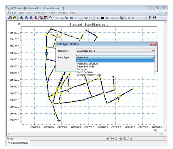
When selecting using the map, the user should directly select the grid-point on the link which should be plotted. The same method as used when selecting results in MIKE URBAN.
