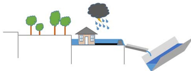
Figure 30.10 Conceptualization of the overland drainage function
