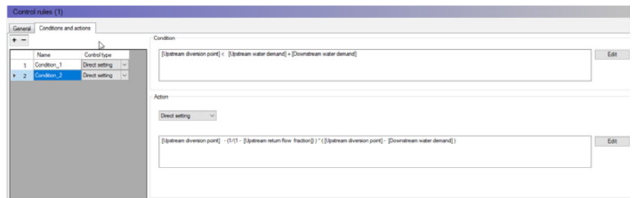
Figure 16.5 Control rules editor, Conditions and Actions tab
