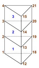
The element table for a mesh of prismatic elements will consist of 6 nodes and for hexahedra of 8 nodes. Example from the figure above:
