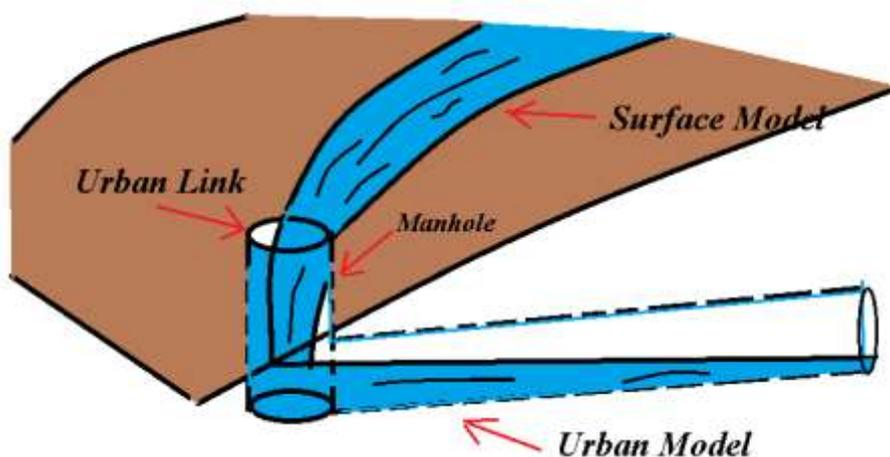
Figure 8: Illustration of a representative urban link (manhole)
