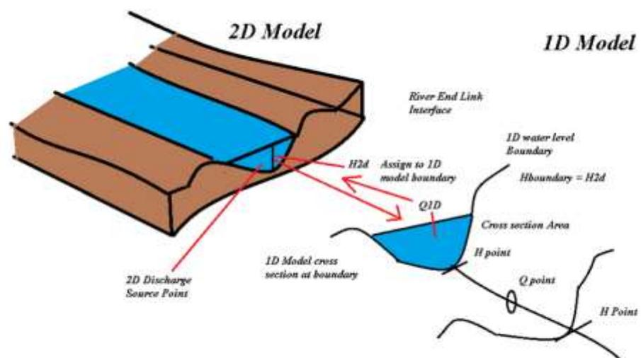
Figure 1: Conceptual diagram of a River End link
