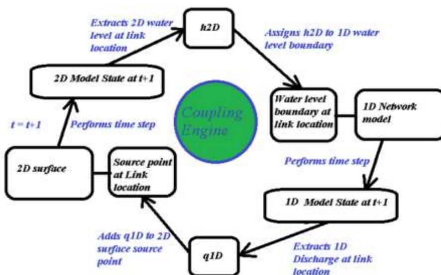
Figure 2: Conceptual diagram of the calculation sequence at a River End or Urban Outlet link
