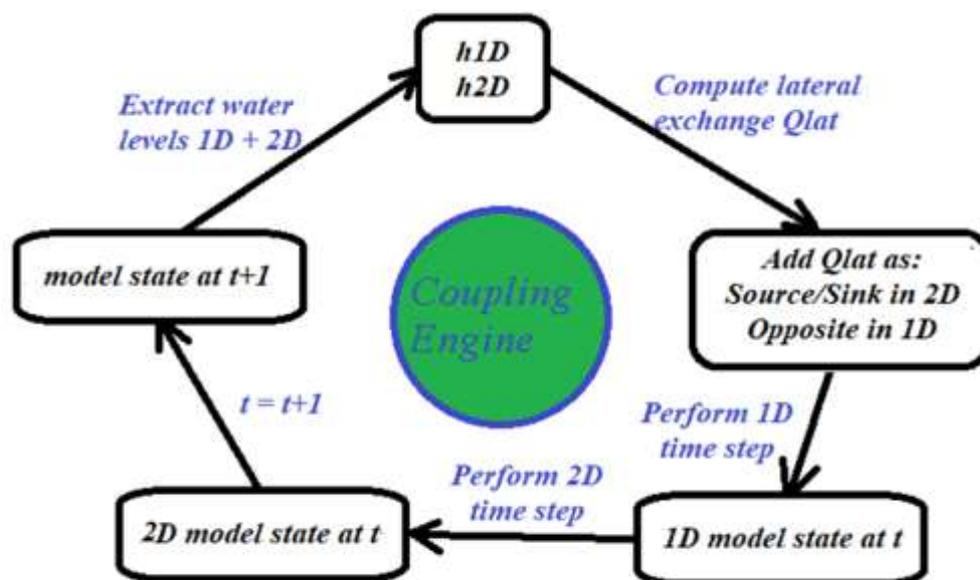
Figure 6: Conceptual diagram of the calculation sequence at a Lateral link
