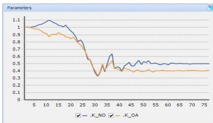
Figure 11.4 Progression of the estimated values for K_NO and K_OA during the Parameter Estimation experiment
