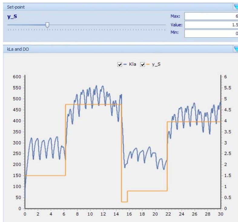
Figure 8.12 Movement of the slider for the manipulated variable y_S (top) and its effect on the actual aeration via kLa (bottom)
