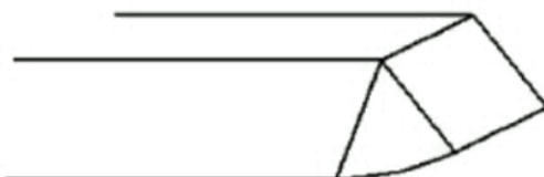
Figure 3.77 Definition sketch of opening type III (sloping embankments and sloping abutments; spillthrough) (after Matthai)
