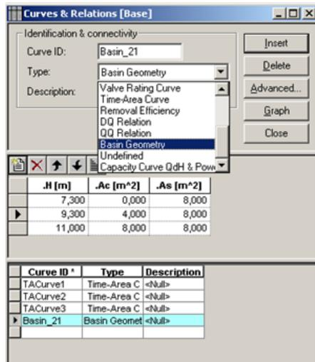
In MOUSE/'Nodes and Structures' select the created basin in the list and under 'Basin Geometry' choose the basin geometry.
