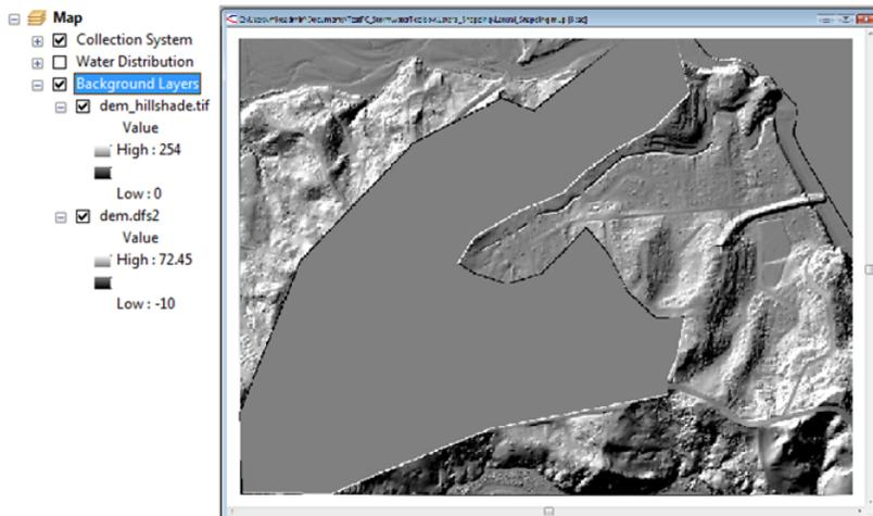
3. Zoom in to the lower-right area of the map where a road could be recognized from the “dem\_hillshade.tif” raster as shown in the figure.
