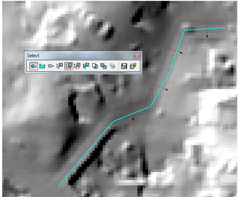
Note that the tool will generate CRSs for the selected links. If no particular links are selected, the tool will generate CRSs for all links intersecting existing cross section lines.
