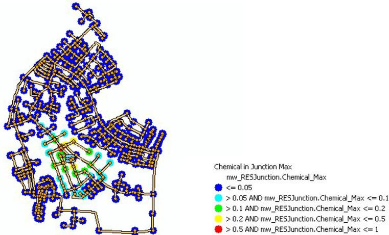
Figure 6.90 Maximum chlorine concentration at each junction node
