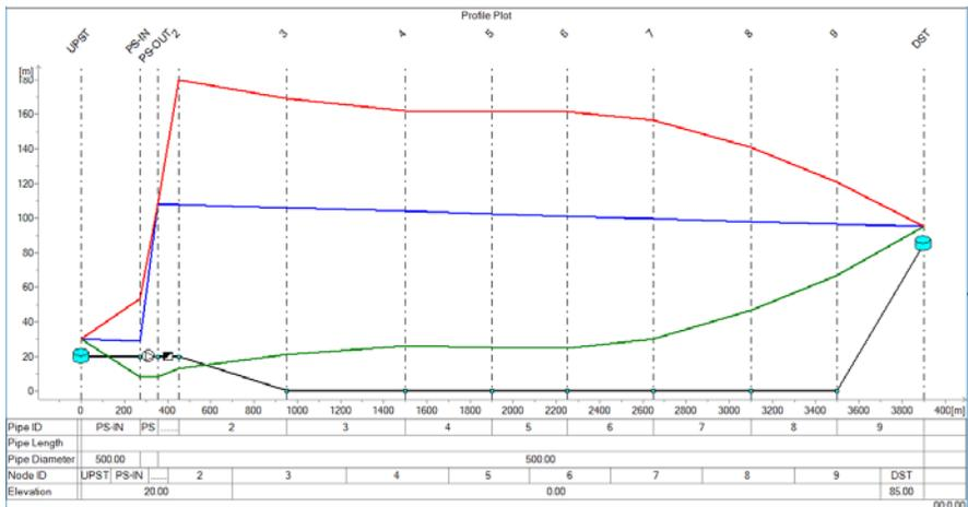
Figure 6.112 Profile plot with HGL levels
