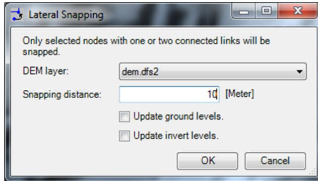
9. The selected nodes are then snapped to the lowest point in the DEM within a lateral distance of 10 m.
