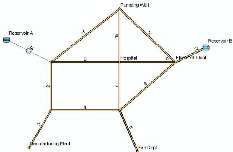
Figure 6.1 A schematic diagram of the pipe network system used in this lesson
