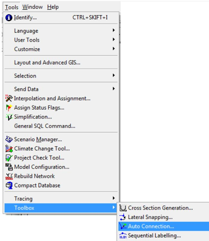
3. Specify the settings for the Auto Connection tool. Select “OL” for the “From nodes” and “Storm Water” for the “To nodes” to generate connections going from the overland to the underground network.
