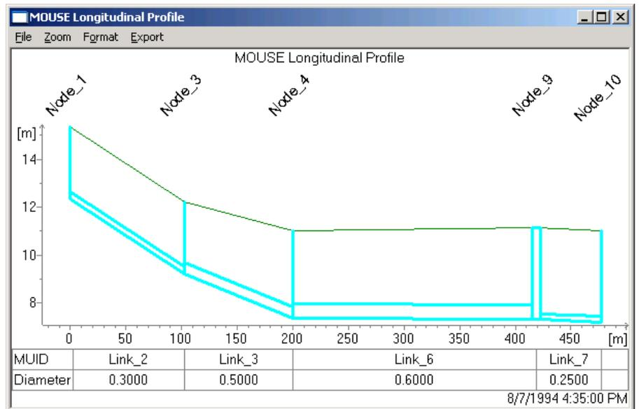
If results are loaded in, the longitudinal profile will be appearing with results added to the profile plot. For a MOUSE result file the water level will be added per default. If you wish to show other results or change the layout of the profile go to the profile plot properties dialog (right-click on the profile to get to the local menu that provides easy access to the property page).
