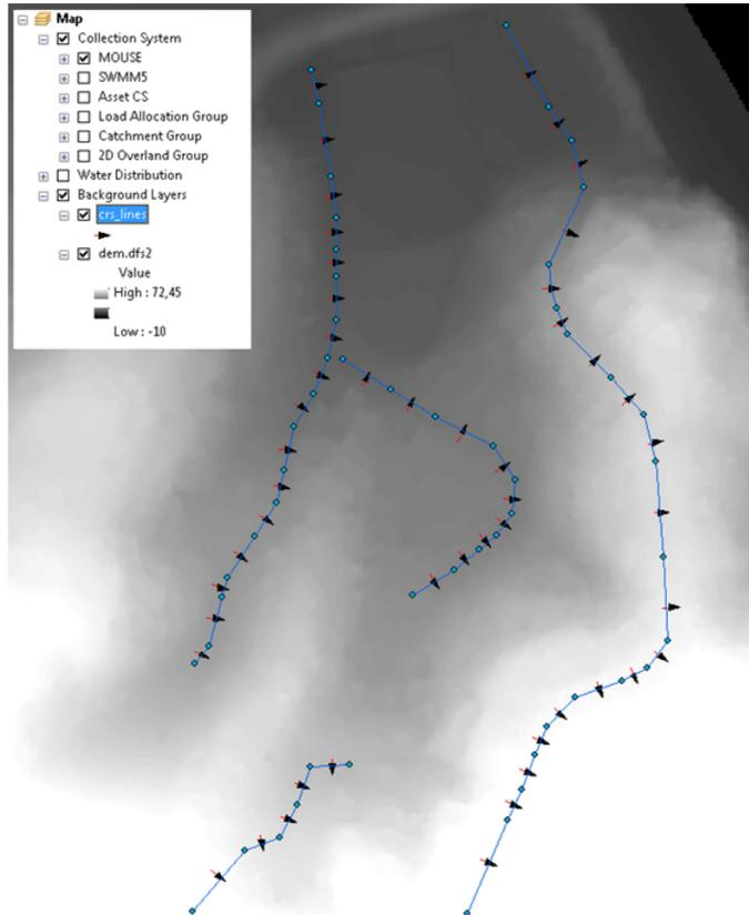
The cross section lines “crs\_lines.shp” are polyline features that were created in ArcMap. They represent estimated alignments and widths of cross-sections for overland channel segments.
