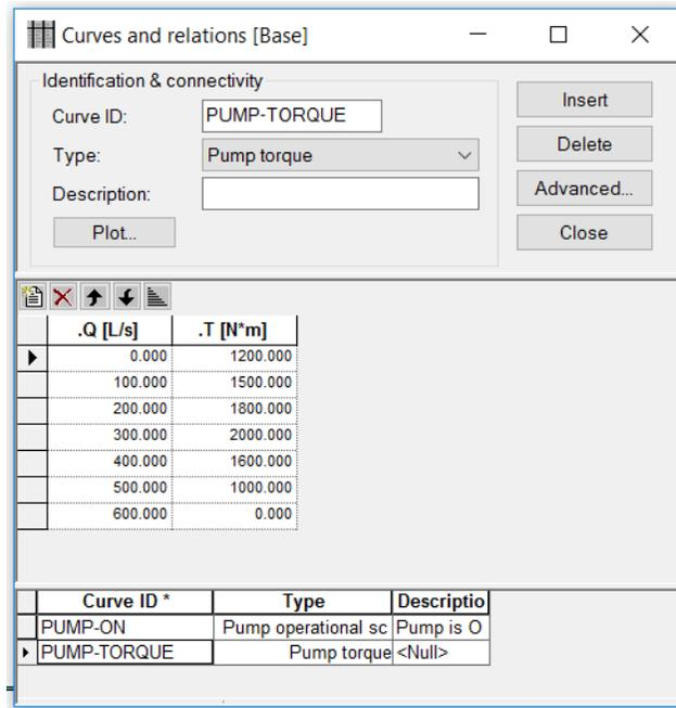
Figure 6.109 Curves data (pump torque)
