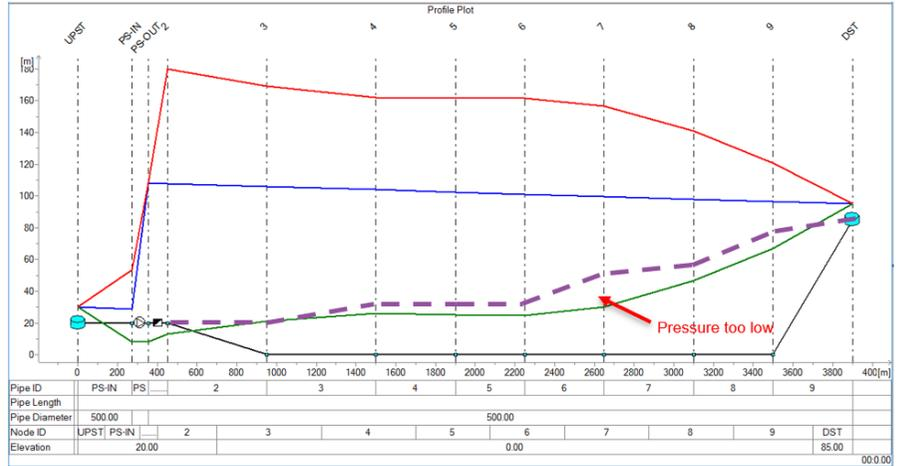
Figure 6.113 Profile plot with HGL levels and potential or future pipeline elevation
