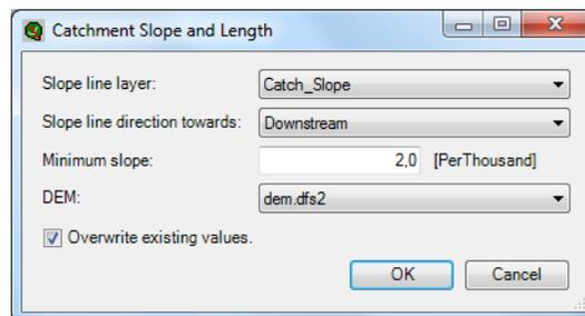
Choose the “Catch\_Slope.shp” layer as the “Slope line layer.” The slope line direction is towards the downstream. A minimum slope can be specified. If the calculated slope is less than the specified minimum slope then this minimum slope value is used. Finally, select the “dem.dfs2” file as the DEM layer for the calculation of the slope and length.
