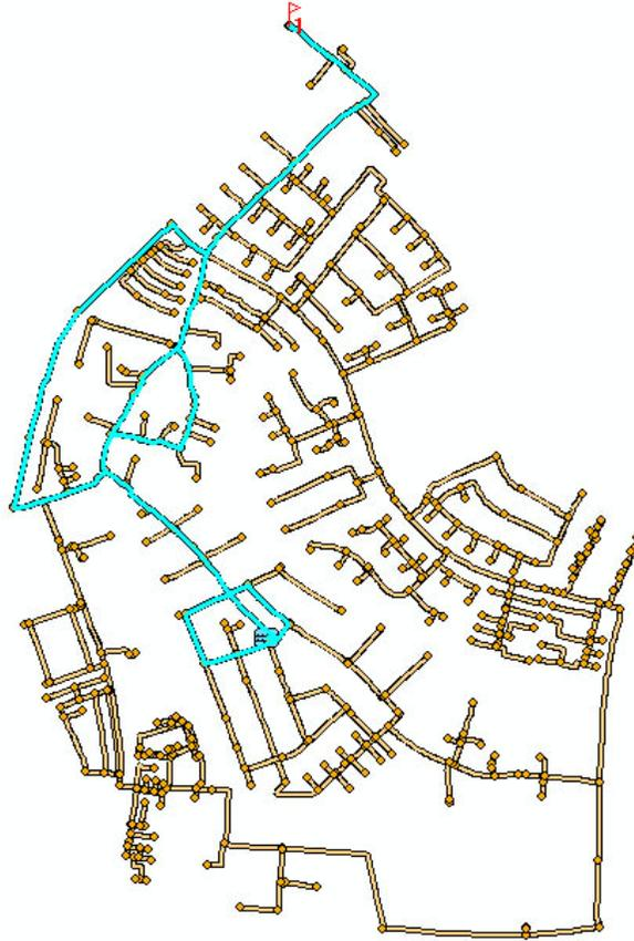
Figure 6.63 Backward tracing of water to junction node 11498
