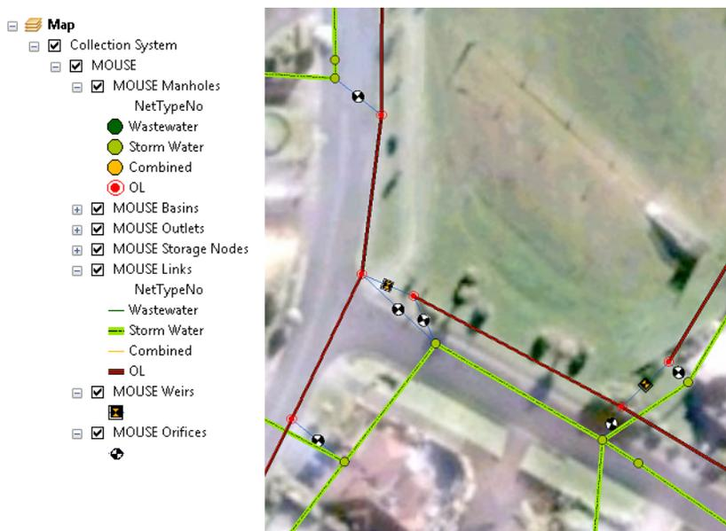
The green network represents the underground Storm Water network and the red network represents the Overland flow network. The overland network is connected to the stormwater network by orifices while the overland network elements are connected to each other by weirs.
