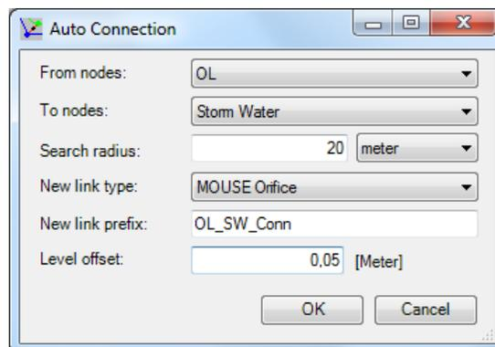
Setting the network type for the “From nodes” and “To nodes” gives more control over the setting-up of connections and also defines the direction of positive flow (From “From nodes” to “To nodes”). For connections from the overland to the underground network the positive
