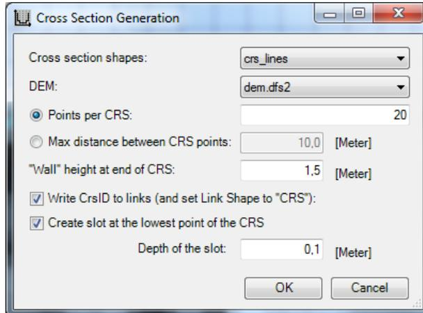
Add side walls to the CRS being generated through the “Wall height at the end of CRS” parameter. This will avoid a MIKE URBAN network simulation to stop if the water level in an open channel rises above the defined CRS height. Use a side wall of 1 to 2 meters for an overland flow path such as a road, and 3 to 5 meters for waterways. Adding side-walls adds 2 points to the number of CRS points specified in the tool.
