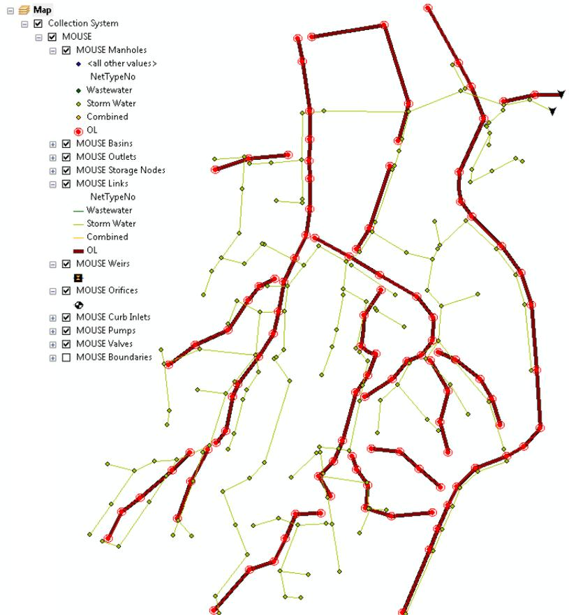
Information about the network type can be found in the “Network type” and “Description” parameters of nodes and links.
