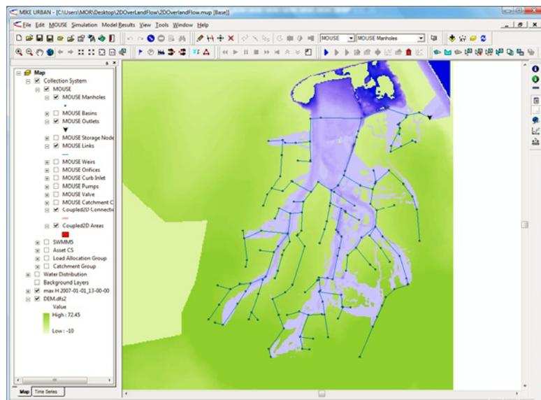
Figure 5.1 The model with DEM and flooding results
