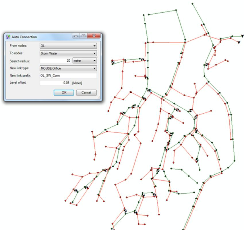
Check the new connections that have been generated by opening the “Orifices” editor through “MOUSE | Orifices”.
