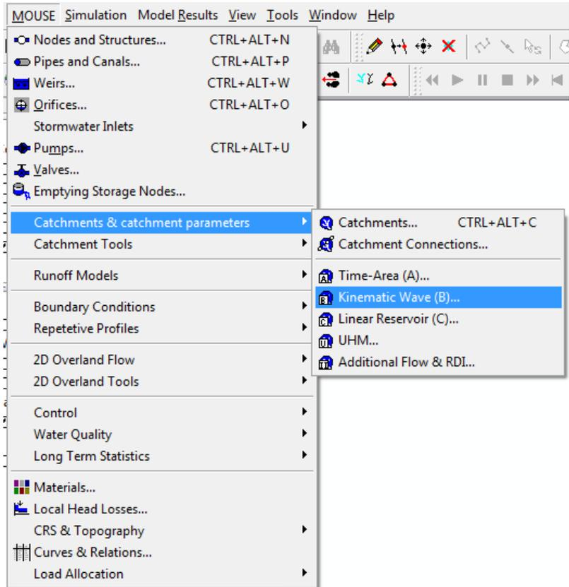
If the Kinematic Wave (B) parameters table is empty, generate records by clicking on “Advanced | Generate model records.” This will generate Kinematic Wave (B) parameter records for all the catchments listed in the Catchments table.
