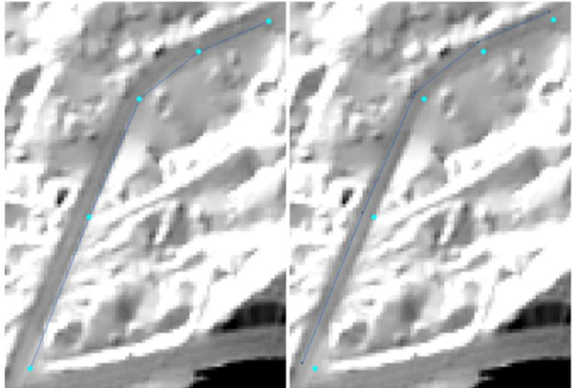
10. In the Lateral Snapping tool dialog, you may choose to update either the node ground levels or the invert levels. For overland flow path (e.g. street network) nodes, the “Update invert levels” would be more appropriate, while for underground stormwater network nodes the “Update ground levels” option is more fitting.
