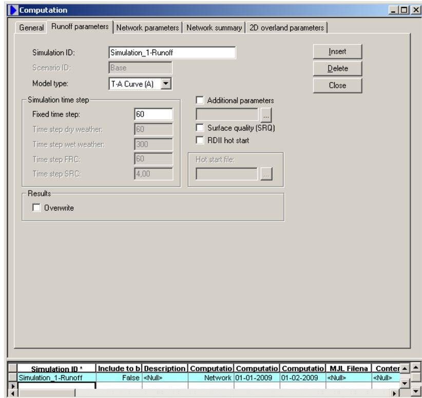
Return to the General TAB and press 'Start Simulation'. The system starts with export of model data to MOUSE.
