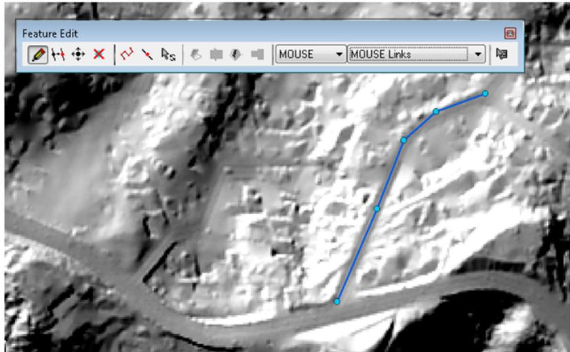
6. To begin using the Lateral Snapping tool, select the newly created nodes that were generated with the new link features. Note that only the nodes should be selected.
