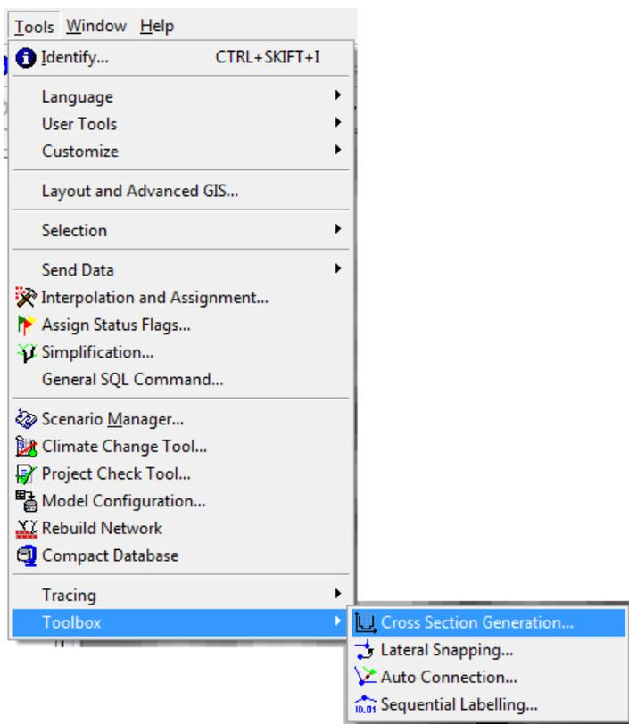
5. Specify the parameters for the Cross Section Generation tool. Choose the cross section alignment layer "crs\_lines" for "Cross section shapes". Choose "dem.dfs2" for "DEM". Specify the number of sample points at which the cross section will be extracted (i.e. 20). Alternatively, you may specify the sample point distance.
