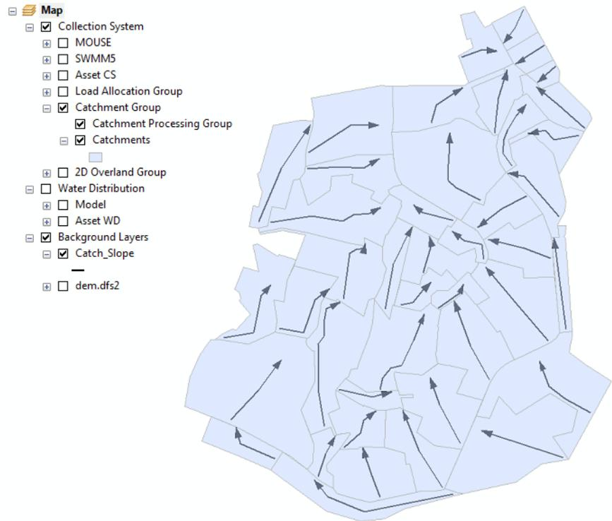
Flow paths can be drawn from the load point or towards the load point but a consistent methodology should be used in a project. A multiple number of slope lines can be defined for each catchment and the slope and length is calculated as an average slope and length of all lines completely within the catchment.
