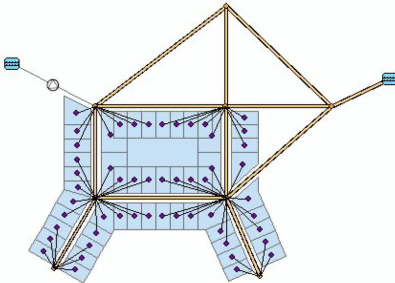
Figure 6.102 Demand points are geocoded to nodes
