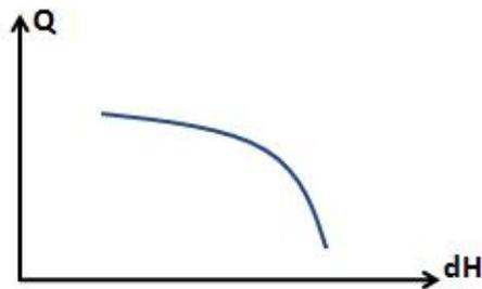
Figure 3.23 Typical example of pump curve
