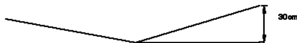
Figure 4.14 Side view of a V-formed levee. The V-form ensures that water gradually flows over the levee.
