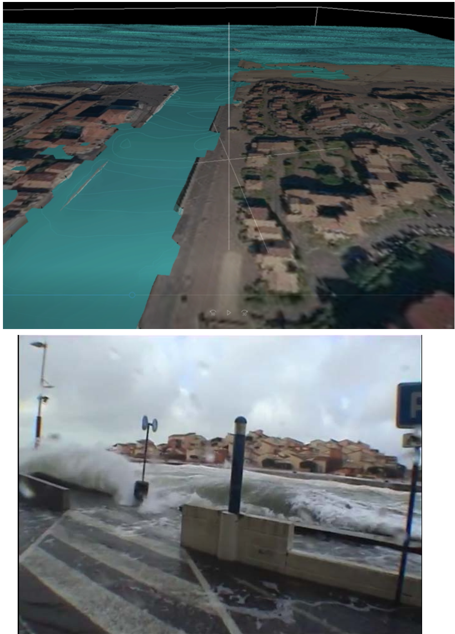
Figure 4.23 Wave overtopping in Capbreton harbour. Upper panel shows a 3D picture of the simulated instantaneous surface elevation in Capbreton entrance channel. Lower panel shows a screenshot of a video taken during the storm on the southern quay of the entrance channel (Source: YouTube, Mars 2014, retrieved from http://www.youtube.com/watch?v=6YuNtXfUHMM )
