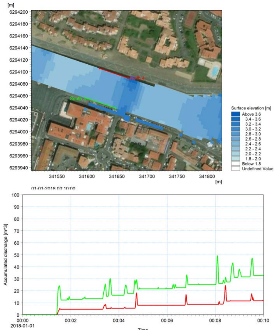
Figure 4.24 Upper panel shows a "zoomed-in" view of Figure 4.22 in the entrance channel with the location of two discharge output lines along the quays. Lower panel shows time series of the accumulated discharges across these lines over the duration of the simulation.
