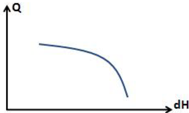
Figure 3.23 Typical example of pump curve
