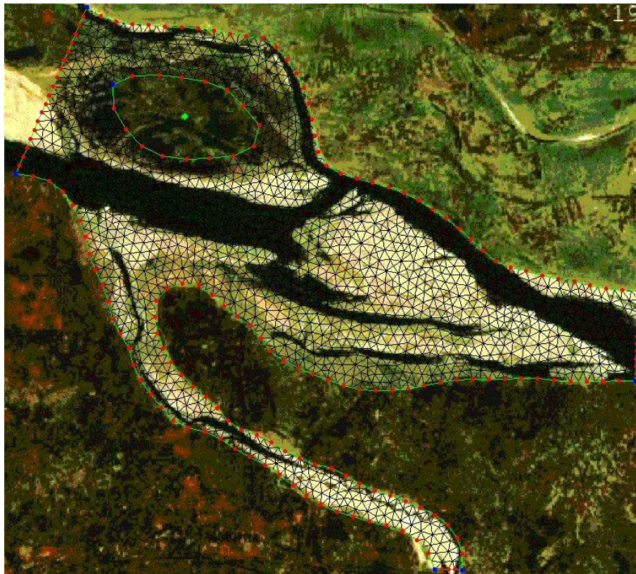
Figure 2.4 Digitised boundaries and generated mesh
