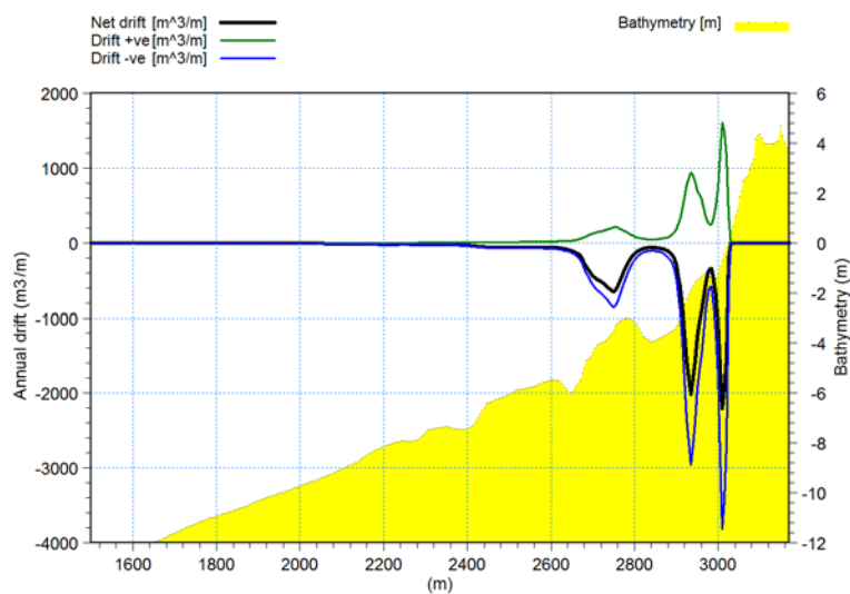
Figure 3.10 Cross-shore distribution of net littoral drift along with the related upstream and downstream components (detail of profile)
