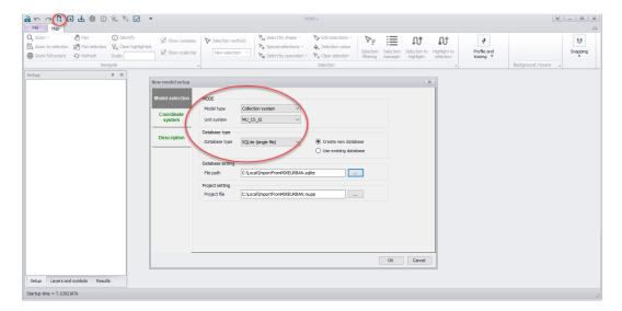
Select the model type and unit system as desired. Also select a database type: the SQLite format is the default format, for use with a local database file.
