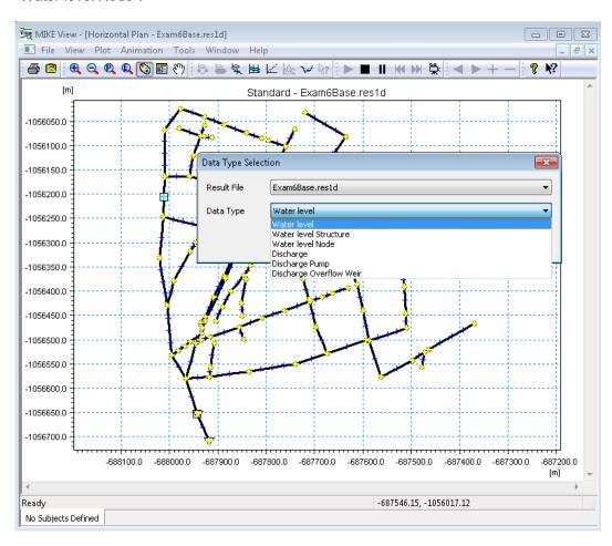
When selecting using the map, the user should directly select the grid-point on the link which should be plotted. The same method as used when selecting results in MIKE URBAN.
