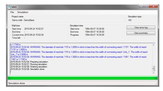
Under the menu "File | Load Simulation" or "File | Load Simulation from GDB folder" it is possible to load a database and rerun a simulation. If several simulation parameters exist in the selected database, the latest run simulation will be re-run.
