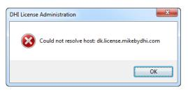
This error message indicates a network connection or configuration error. The PC is not able to resolve which address is behind "dk.license.mikebydhi.com".
