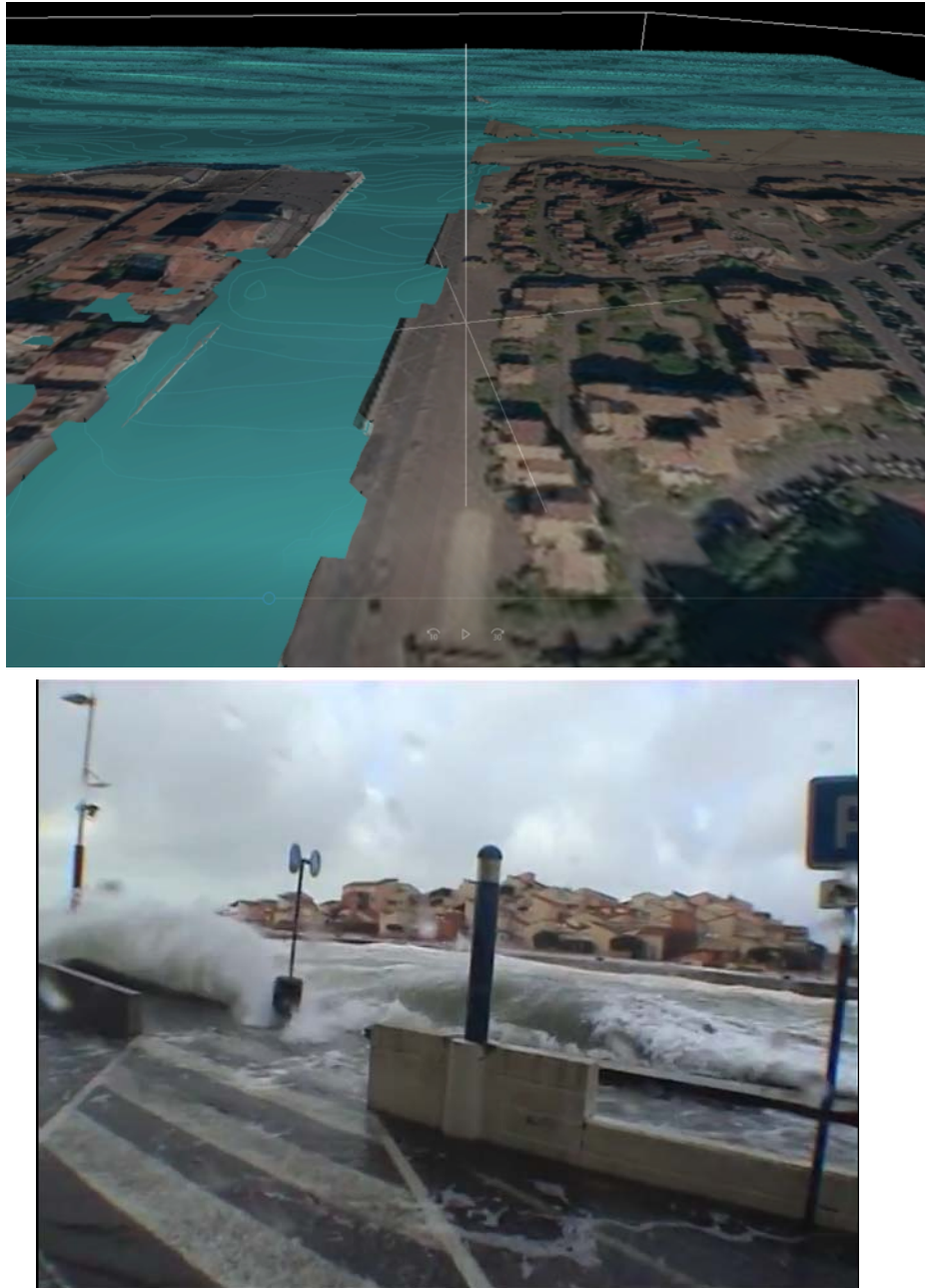
Figure 4.21 Wave overtopping in Capbreton harbour. Upper panel shows a 3D picture of the simulated instantaneous surface elevation in Capbreton entrance channel. Lower panel shows a screenshot of a video taken during the storm on the southern quay of the entrance channel (Source: YouTube, Mars 2014, retrieved from http://www.youtube.com/watch?v=6YuNtXfUHMM )
