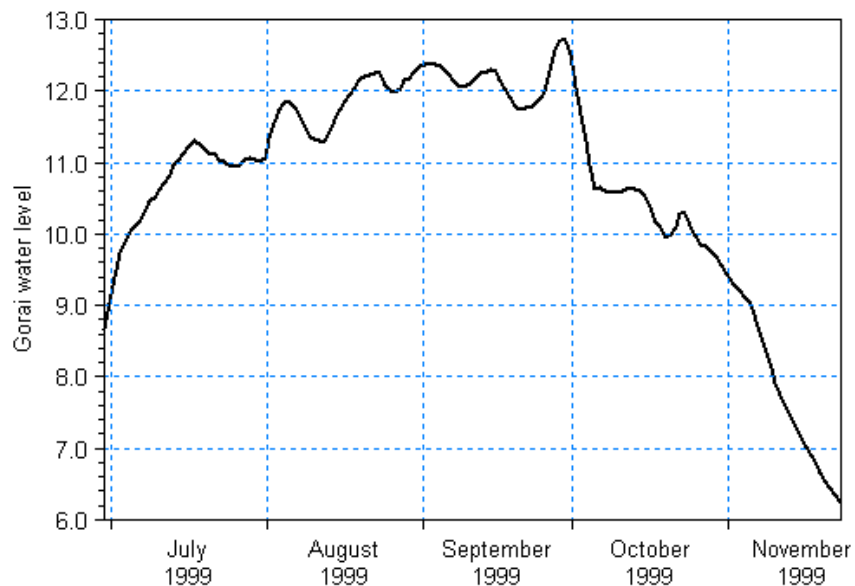
Figure 3.4 Gorai water level variation applied as downstream boundary condition for the simulation of the 1999 monsoon
