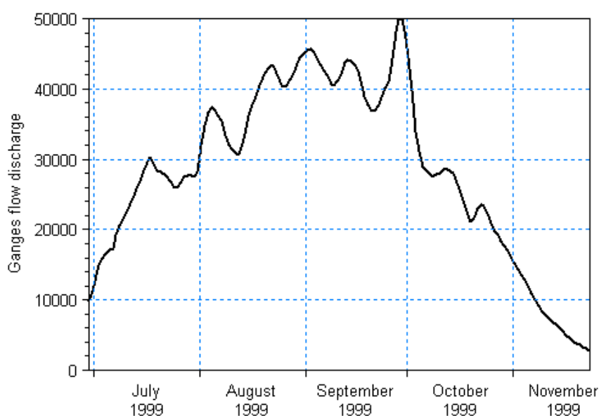
Figure 3.2 Rated flow discharge applied at the upstream Ganges boundary for the 1999 monsoon
