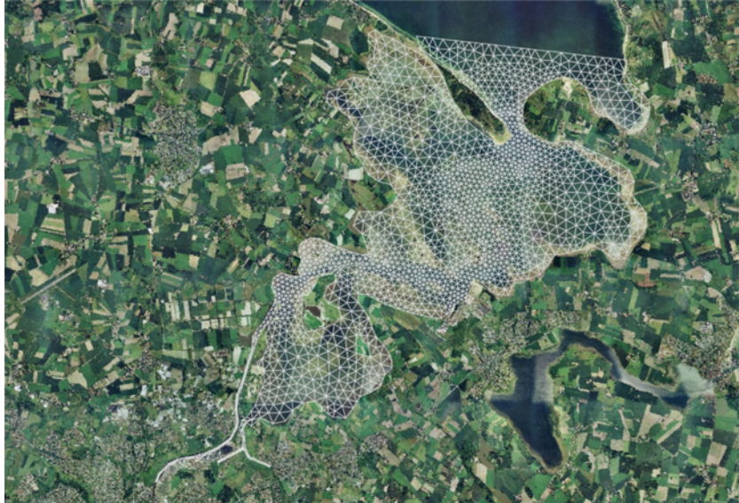
Figure 2.1 Odense Estuary, Denmark. Computation mesh used in MIKE 3 Flow Model FM for studying hydrodynamics and ecosystem dynamics.
