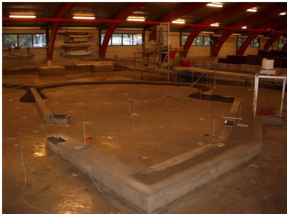
Figure 6.1 Physical model of the Kirkwall Marina
