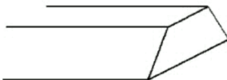
Figure 6.24 Definition sketch of opening type II (sloping embankments without wing-walls) (after Matthai)
