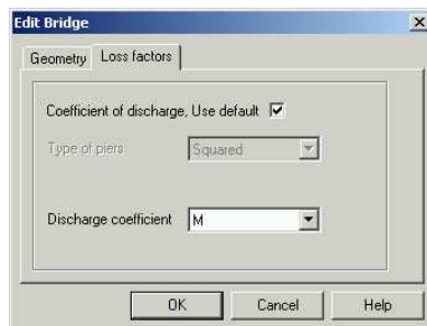
Figure 2.69 Arch Bridge Loss factor property page
