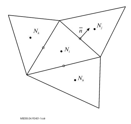
Figure 4.1 • centroid point and  $\circ$  midpoint of edges
