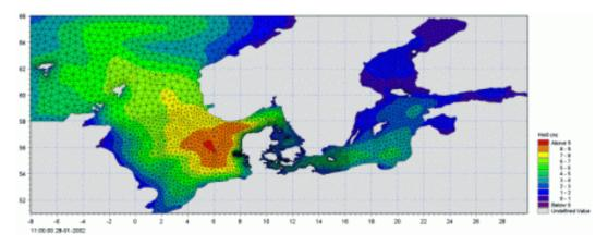
Figure 2.1 A MIKE 21 SW forecast application in the North Sea and Baltic Sea. The chart shows a wave field illustrated by the significant wave height in top of the computational mesh
