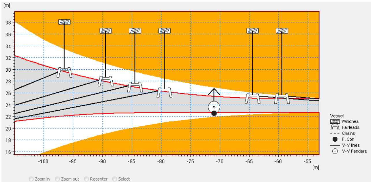
Figure 4-12 Example of a newly defined fender connection (dotted white circle with arrow icon showing the fender force direction)
