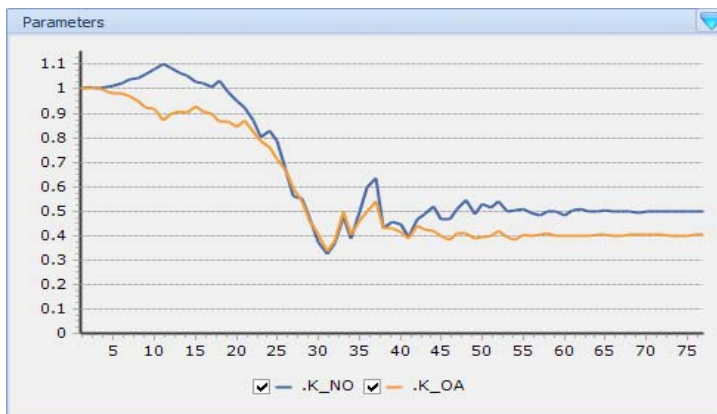
Figure 10.4 Progression of the estimated values for K_NO and K_OA during the Parameter Estimation experiment
