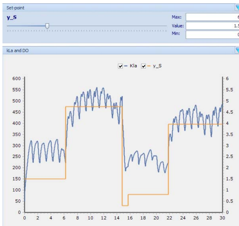
Figure 7.12 Movement of the slider for the manipulated variable y_S (top) and its effect on the actual aeration via kLa (bottom)
