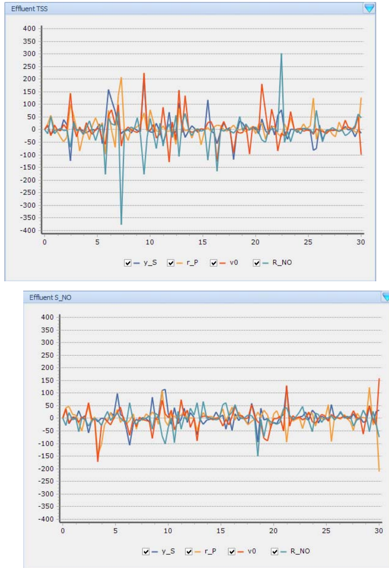
Figure 8.6 Example of plot output for the Local Sensitivity Analysis experiment: Central Relative Sensitivity (CRS) for TSS (top) and Nitrate concentration (bottom) in the effluent
