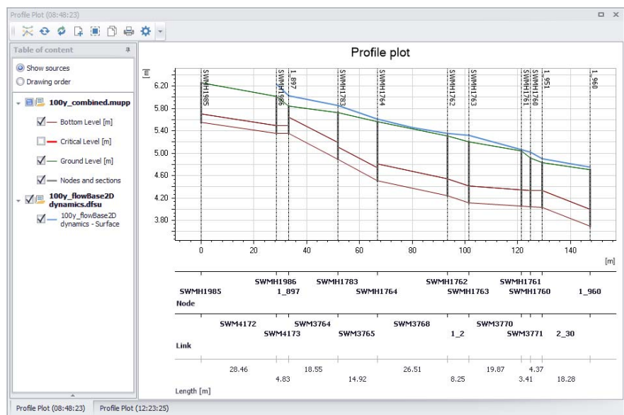
Figure 20.39 The Profile Plot form window showing an example longitudinal profile plot 2D water level simulation results (blue line)
