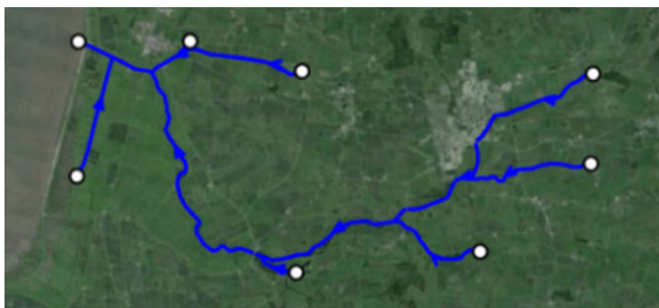
Figure 12.1 River network with 'Open end' boundary locations (black circles)
