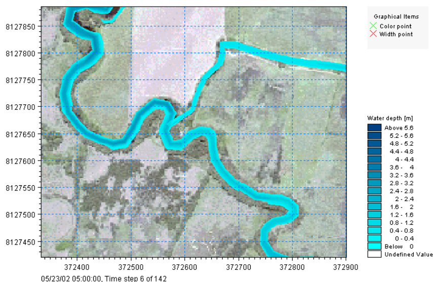
Figure 15.2 An example of a 2D flood inundation map presented in the Result Viewer
