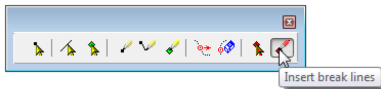
Figure 8.11 Inserting a break line from the Boundary Definition toolbar. Note that you have to be in arc editing mode for the toolbar to activate
