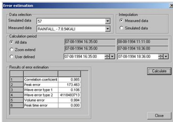
Figure 5.12 An example a corresponding “Error estimation dialog”
