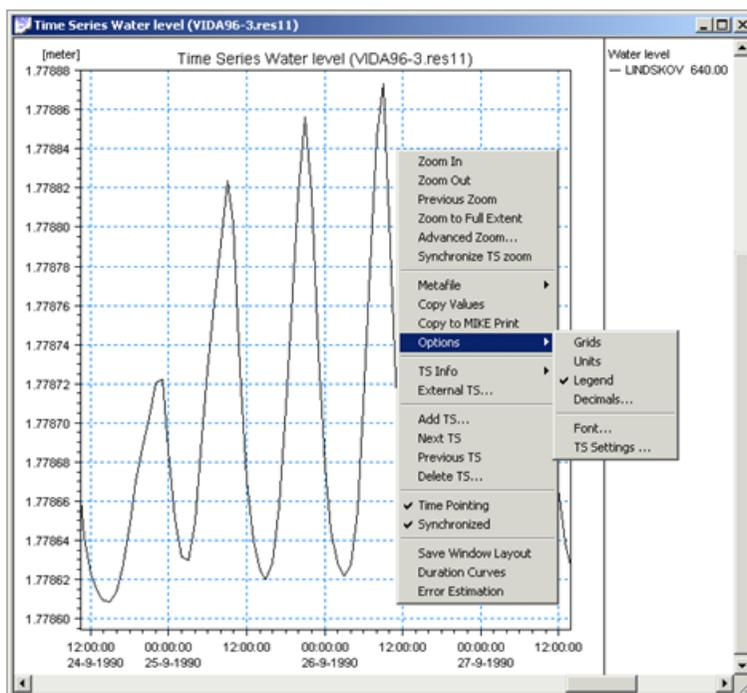
Figure 13.11 Typical Time Series Plot Showing Local Menu Options
