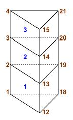
The element table for a mesh of prismatic elements will consist of 6 nodes and for hexahedra of 8 nodes. Example from the figure above:
