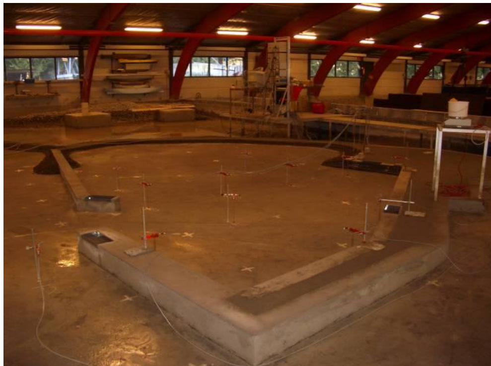
Figure 6.1 Physical model of the Kirkwall Marina
