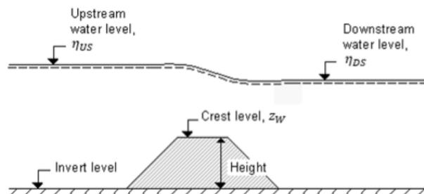
Figure 3.34 Definition sketch for Weir Flow
