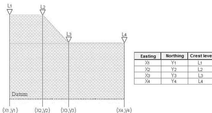
Figure 3.25 Definition sketch of spatial varying dike geometry
