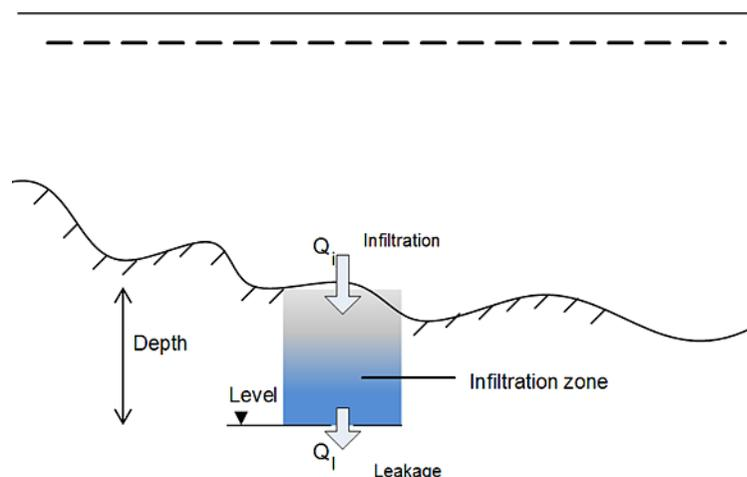
Figure 4.41 Definition of infiltration with storage and leakage: In the case of net infiltration,  $Q_{infiltration} = Q_{leakage}$ , the model assumes an infinite storage volume in the infiltration zone.
