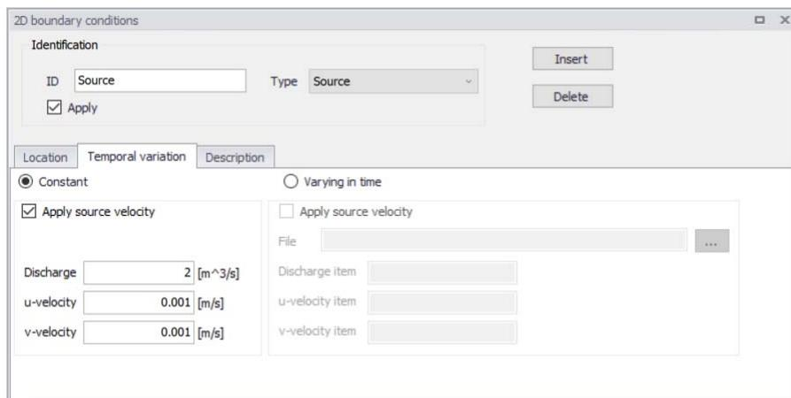
Figure 4.15 Temporal Variation tab for Source 2D boundary conditions
