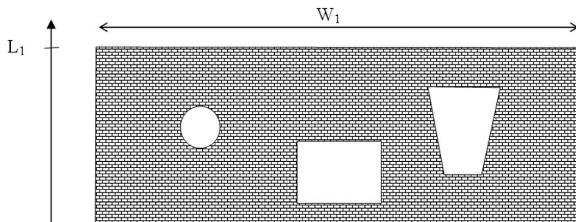
Figure 3.37 Wide weir with multiple culvert openings
