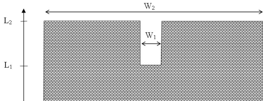
Figure 3.36 Wide weir with a small opening
