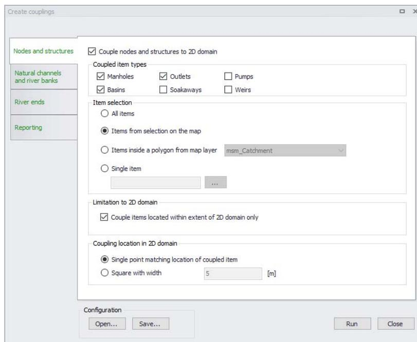
Figure 5.3 Create couplings tool - couple Nodes and structures
