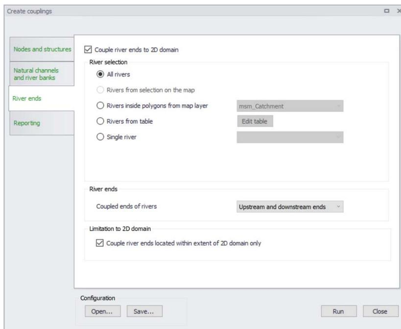
Figure 5.7 Create couplings tool - couple River ends
