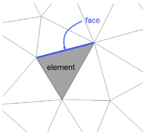
Figure 3.24 Illustration of elements and element faces
