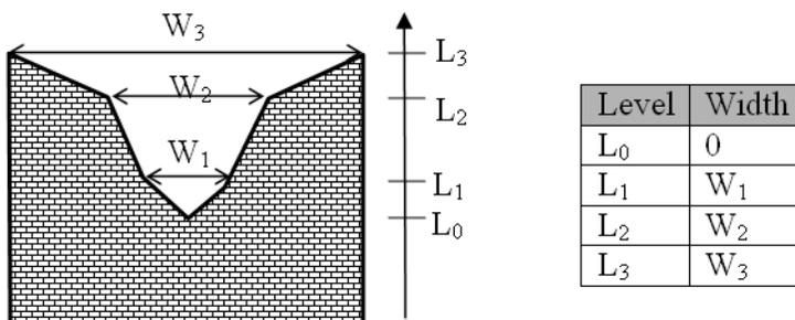
Figure 3.33 Definition sketch of broad crested weir geometry
