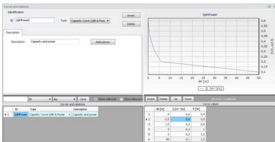
Figure 7.5 Pump capacity curve including power consumption
