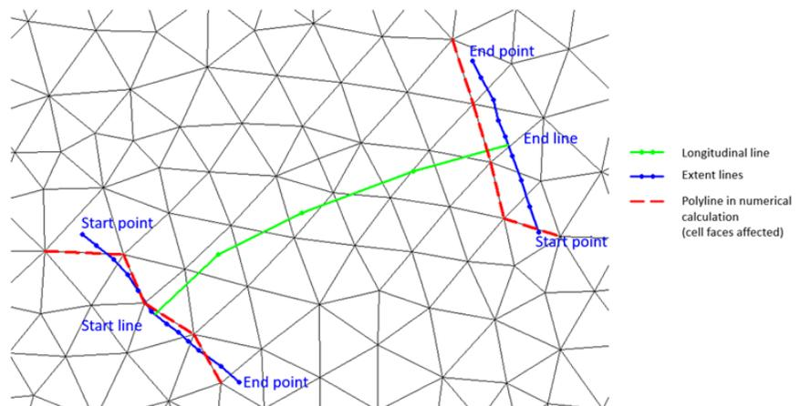
Figure 3.28 Definition sketch for a long culvert
