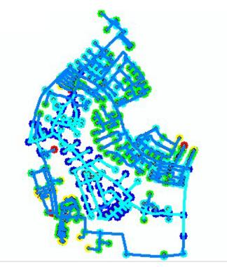
Figure 6.77 Maximum water age at each junction node
