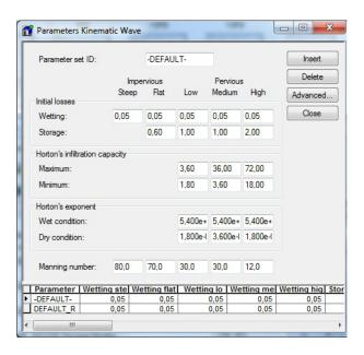
Figure 4.8 The Kinematic Wave Parameter Sets Editor (MOUSE|Runoff Models|Parameters Kinematic Wave)
