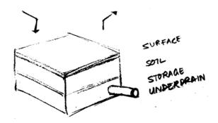
Figure 4.22 Bio retention cell structure layers
