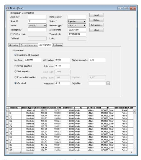
Figure 8.13 2D Overland flow tab in the nodes dialog
