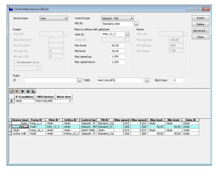
Figure 9.12 Dialog with control data specific for weirs
