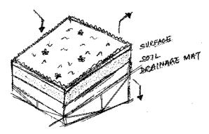
Figure 4.28 Green roof process layers
