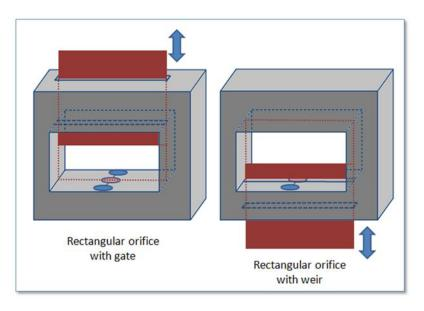
Figure 3.17 Examples on a rectangular orifice with a gate and a weir
