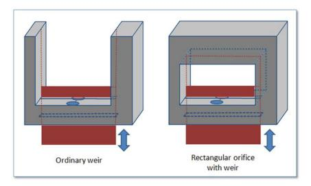
Figure 9.14 Difference between a ordinary weir and an orifice with a weir.
