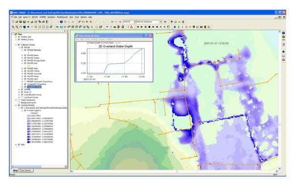
Figure 8.18 2D flood results shown as raster data and time series
