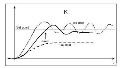
Figure 9.5 Fluctuations around the set point depending on the size of the proportionality factor, K
