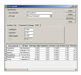
Figure 14.21 The CS SWMM LID Controls Editor - Drain
