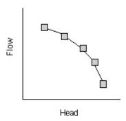
Type 4 - a variable speed in-line pump where flow varies continuously with inlet node depth.
