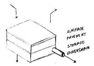
Figure 4.24 Porous Pavement structure layers
