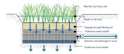
Figure 3.6 Conceptual drawing of a soakaway
