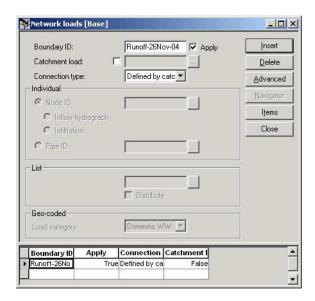
Figure 4.21 The "Network Loads" editor with runoff defined as a load. "Defined by catchment connections" implies that the MOUSE runoff result file (\*.CRF) will be used as a source of connection information
