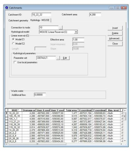
Figure 4.9 The Linear Reservoir Model Editor (MOUSE|Runoff Models|Linear Reservoir (C)), set up for the work with model C1 (Dutch)
