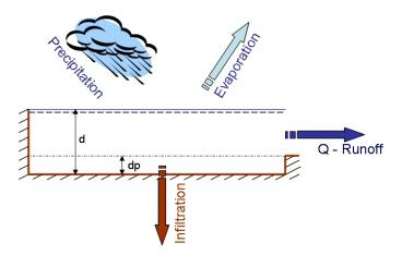
Figure 14.2 Nonlinear Reservoir Concept
