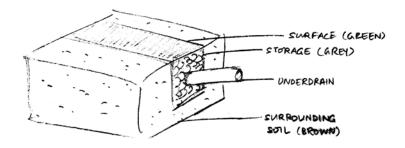
Figure 4.23 Infiltration trench structure layers
