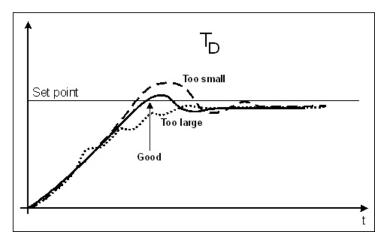
Figure 9.6 Fluctuations around the set point depending on the size of the derivation time, TD.
