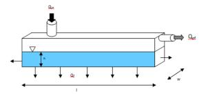
Figure 3.10 Schematic of the soakaway model
