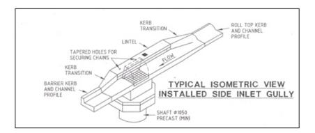
Figure 3.18 A typical curb inlet configuration
