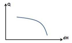
Figure 3.23 Typical example of pump curve
