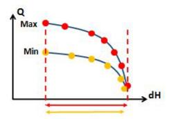
Figure 3.26 The RPMmax and RPMmin pump curves
