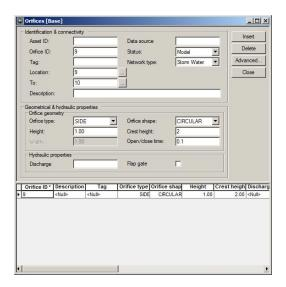
Figure 13.7 The CS SWMM Orifices Editor
