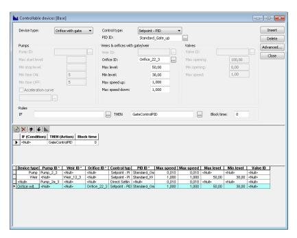
Figure 9.13 Dialog with control data specific for orifices
