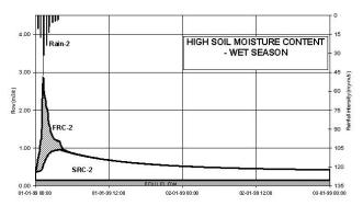
Figure 4.14 Different catchment response under the same rainfall, due to different soil moisture conditions at the beginning of the rainfall
