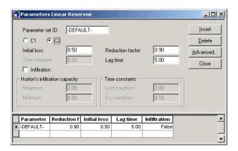
Figure 4.12 The Linear Reservoir Parameter Sets Editor (MOUSE|Runoff Models|Parameters Linear Reservoir) - French version
