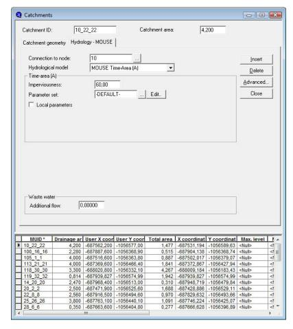
Figure 4.3 The Time-Area Model Editor (MOUSE|Runoff Models|Time-Area (A))
