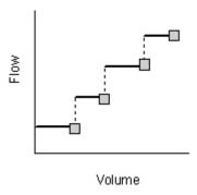
*Type 2* - an in-line pump where flow increases incrementally with inlet node depth.
