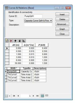
Figure 5.3 Pump capacity curve including power consumption
