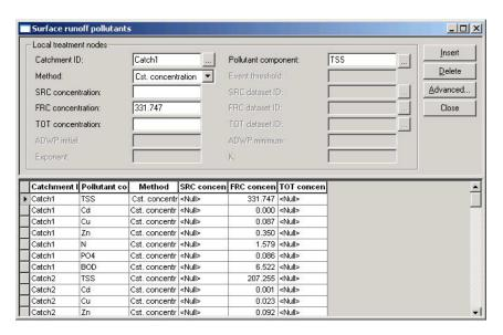
Figure 12.21 Assigning surface runoff pollutants
