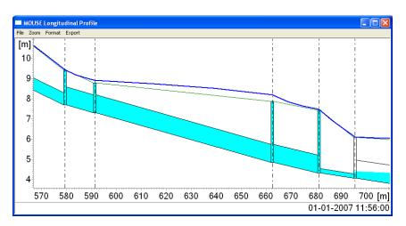
Figure 8.19 2D flood results shown as water surface profile in longitudinal profile
