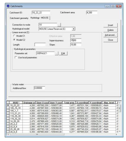
Figure 4.10 The Linear Reservoir Model Editor (MOUSE|Runoff Models|Linear Reservoir (C)), set up for the work with model C2 (French)
