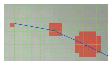
Figure 8.11 Nodes coupled to varying numbers of 2D cells
