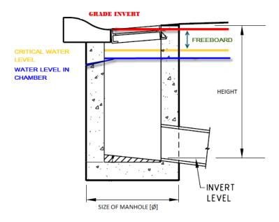
Figure 8.14 Freeboard detail in a Curb Inlet
