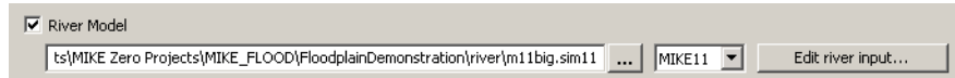
Figure 3.14 MIKE HYDRO River or MIKE 11 simulation file path name along related buttons. Note the tick box on the left which may be used to select or de-select whether a river set-up is to be included.
