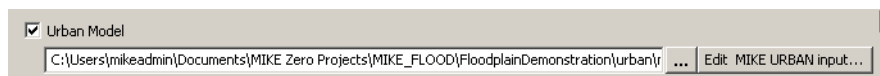
Figure 3.15 MIKE URBAN file path. If a MIKE URBAN database has been selected the ‘Edit MIKE URBAN’ button will be active and the user may access the MIKE URBAN set-up directly
