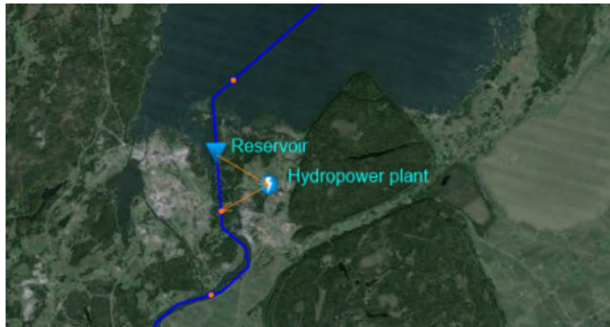
Figure 10.1 Hydropower plant defined with a single reservoir connection and return flow definition to river location downstream of reservoir
