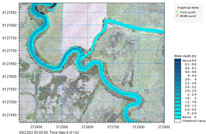
Figure 6.15 An example of a flood inundation map presented in the Result Viewer
