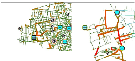
Figure 3.25 Pipe criticality results, Map view (pipes are colour coded by the pipe criticality C)
