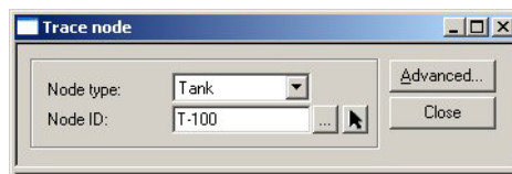
Figure 1.45 The Trace Node dialog box is used to specify a single node that acts like a tracer in determining what percent of its water reaches any other node in the network
