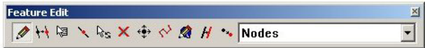
Figure 9.1 Use the Add Node tool for interactively laying out the network manhole nodes in the CS MOUSE mode
