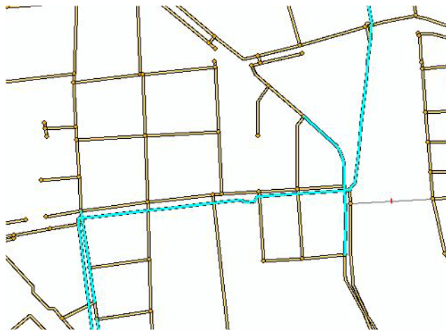
Figure 23.56 Pipes where the flow direction has changed are selected on the Map
