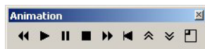
Figure 6.70 Animation allows you to animate the results in time or to select a different time step in which to display results
