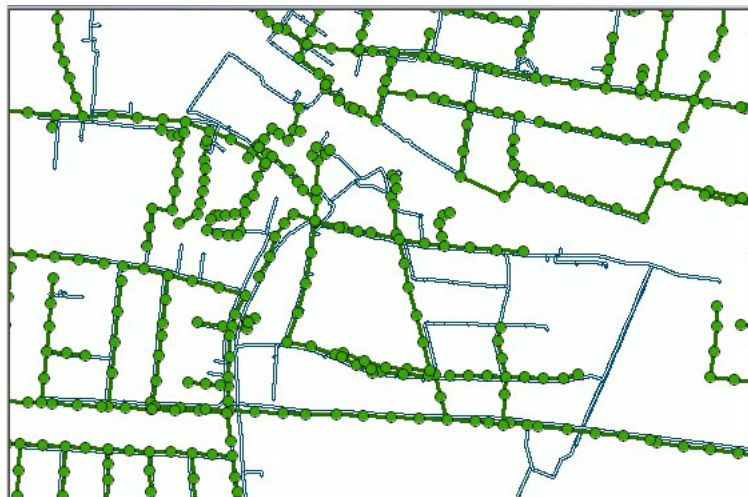
Figure 2.1 The water distribution and sewer network from a major metropolitan city, which is used in the lesson
