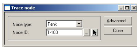
Figure 1.45 The Trace Node dialog box is used to specify a single node that acts like a tracer in determining what percent of its water reaches any other node in the network
