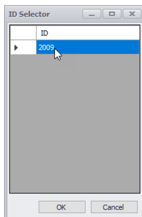
Figure 3.10 Select a TopoID for a river branch from the list of available sets on the ID Selector window accessed via the ellipsis button.
