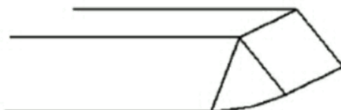
Figure 3.77 Definition sketch of opening type III (sloping embankments and sloping abutments; spillthrough) (after Matthai)
