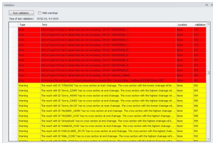
Figure 9.3 The validation list indicates whether an item is an Error (highlighted in red) or a Warning (highlighted in yellow).
