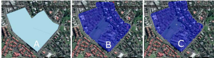
Figure 9.5 The original catchment polygon (A); Edited polygon (blue) with high-lighted vertices; Catchment after completed editing (C).
