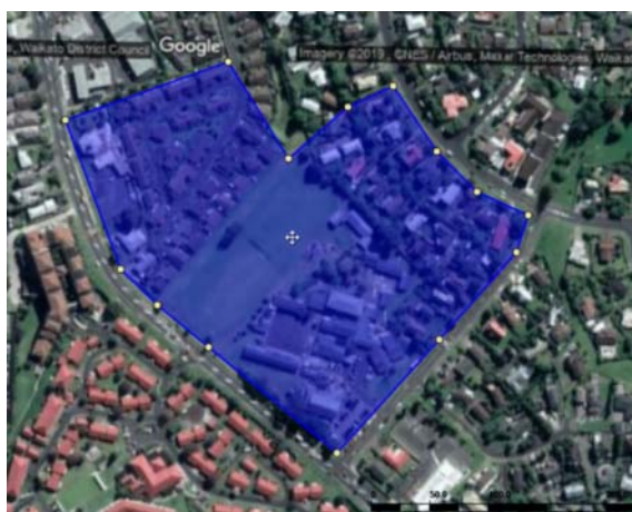
Figure 9.6 Use the crosshairs at the polygon centroid to move the feature during editing.
