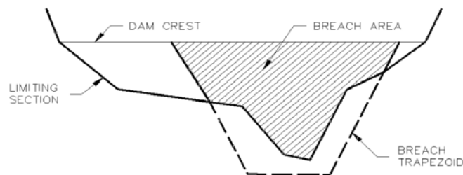
Figure 6.19 The breach (shaded area) is the area of the trapezoid inside the limiting cross section
