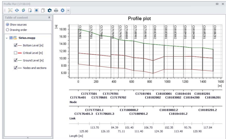
Figure 20.31 The Profile Plot form window showing an example longitudinal profile plot without simulation results
