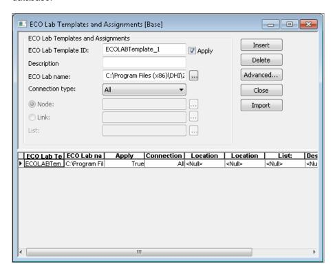
The template can be connected to the hydrodynamic model through nodes or links. The usual options to connect the database are available, all elements, a single link/node or a selection of links/nodes. The "Apply" check box can be used to disable the template.
