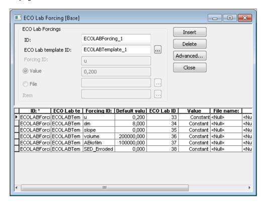
Once the parameters have been defined appropriately in MIKE URBAN, the user is ready to run a MIKE1D Water Quality analysis simulation. In the simulation editor choose MIKE 1D engine as the simulation engine (the old MOUSE engine does not support MIKE ECO Lab analysis), go to the "Network parameters" tab and in the "Pollutants" group tick the Transport AD and the ECO Lab checkbox.
