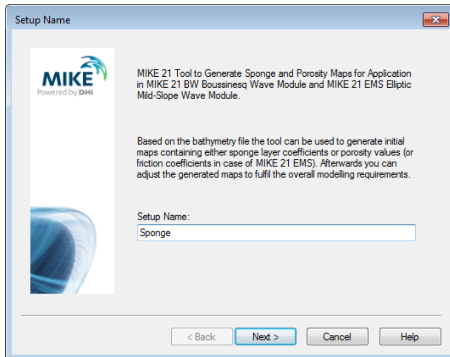
Figure 3.3 Start page of wizard for generation of sponge and porosity layer maps
