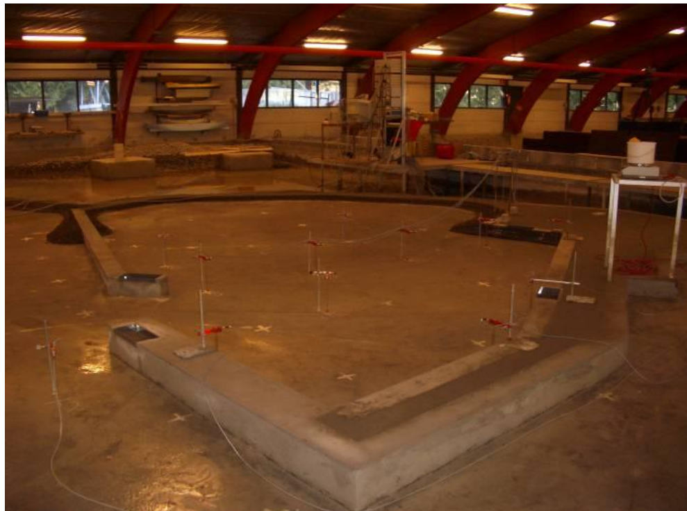
Figure 6.1 Physical model of the Kirkwall Marina
