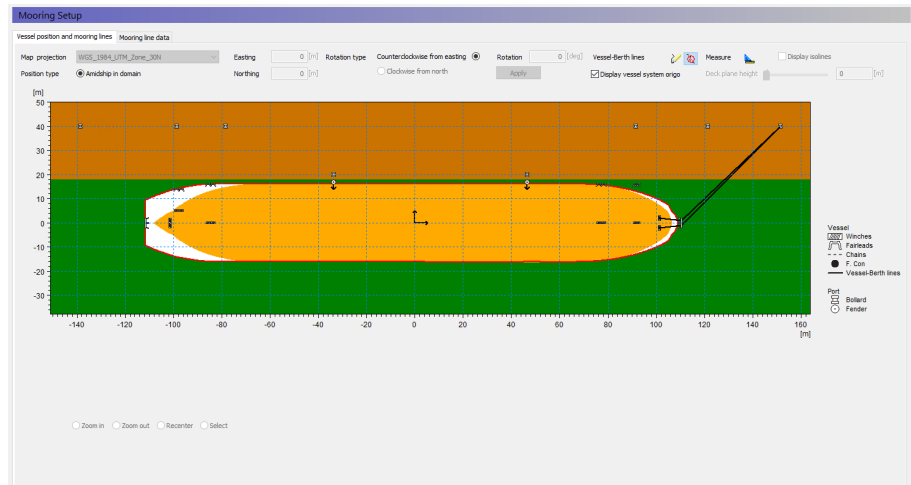
Figure 5.11 Example of inserting mooring lines
